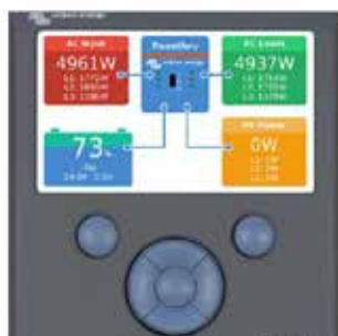
Color Control GX, showing a PV application
